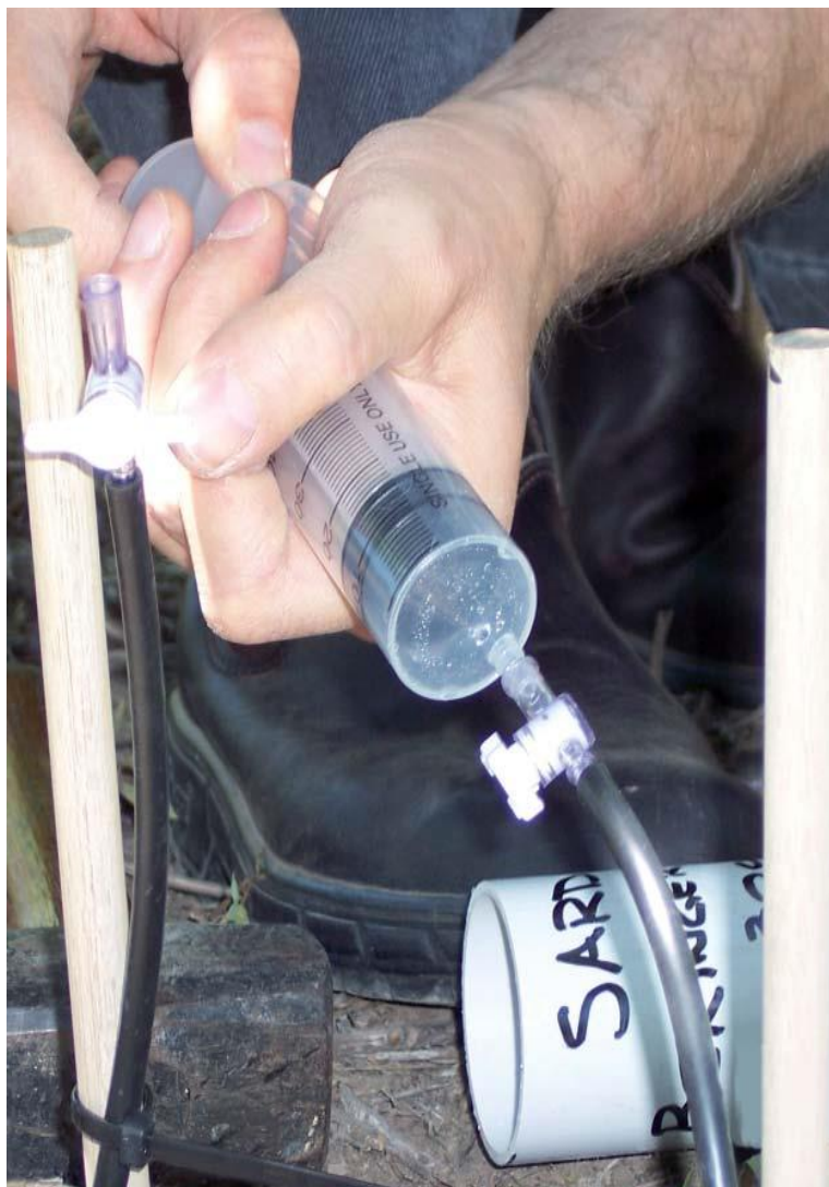
Figure 5. Drawing soil pore water
